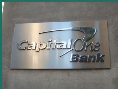
● fabricated polished steel letters over satin plate
